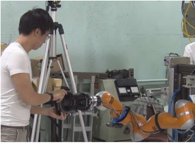
Figure 1: The robot assistant, which utilizes a Kuka Lightweight Robot (LWR) robotic arm mounted to an overhead gantry platform, performs a handover during a car door assembly scenario.
