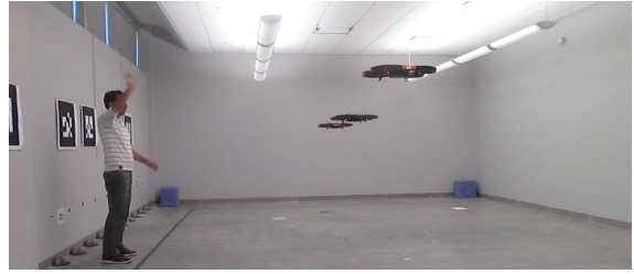
Fig. 3: Exp. 2: Waving gesture interface for HMRS as an example of SSCC method [7].
